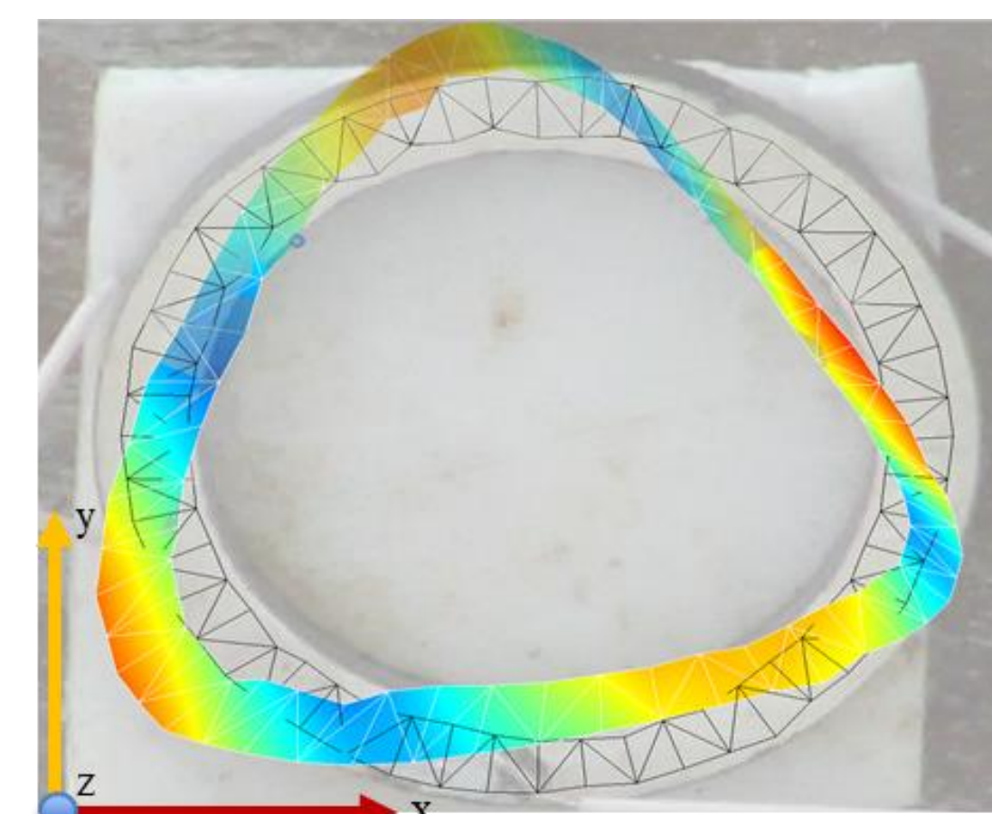
Fig. 4. Deformation mode of the piezoelectric ring at the operational frequency of ~92 kHz
