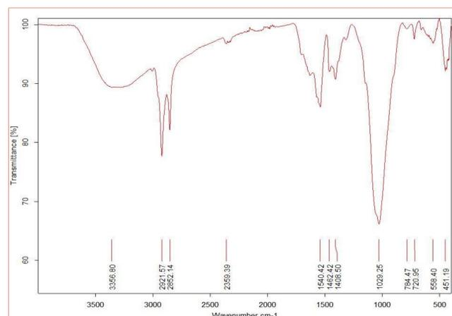
Figure3. FTIR. oleic acid Coated MECNs
