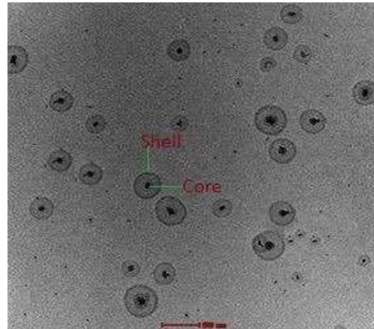
Figure 1. Transmission Electron Microscopy (TEM) image. showing the core shell nanostructure of MECNs ( $\text{Fe}_3\text{O}_4$  Core and Chitosan Shell).
