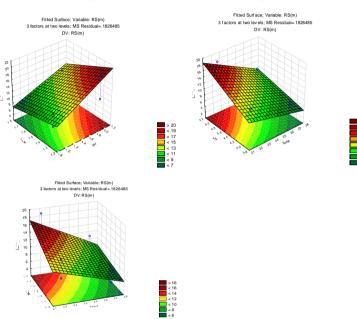
Three dimensional plot for medium resolution variation between FNO, FNS and PHAP at modification with ±10% of pH (4.5), temperature (25 °C), and flowrate (1.5 ml/min)
