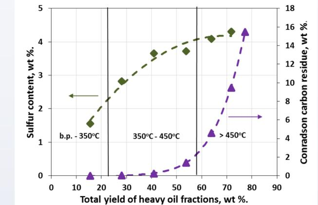
Figure 7. The content of sulfur and CCR of SFEF narrow fractions of heavy oil
