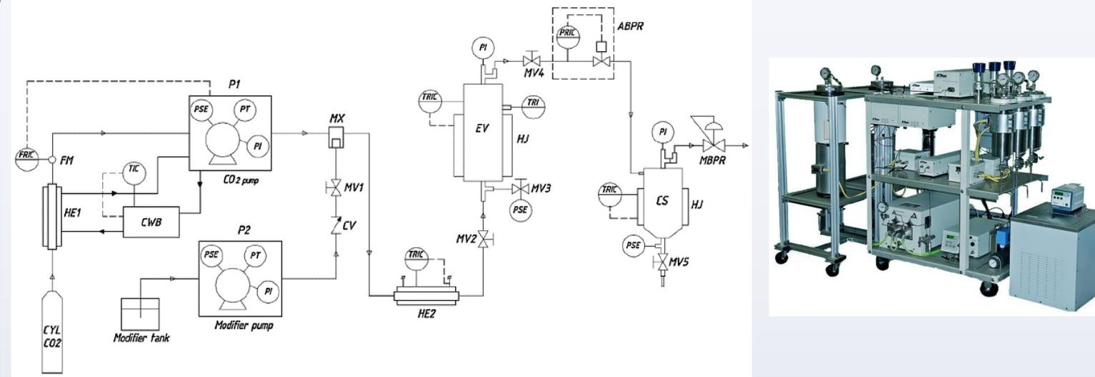
Figure 1. Process flow diagram of the laboratory-scale supercritical fluid extraction and fractionation (SFEF) system
