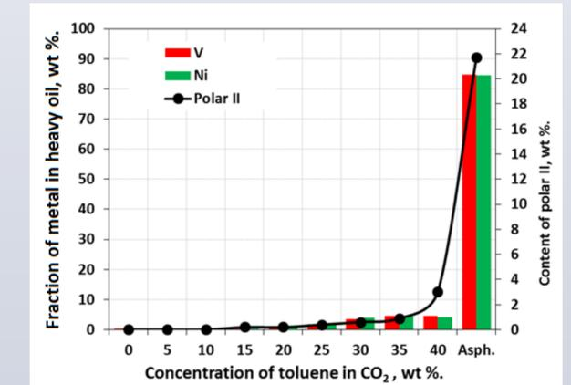
Figure 8. Distribution of metals and content of polar II in SFEF narrow fractions of heavy oil
