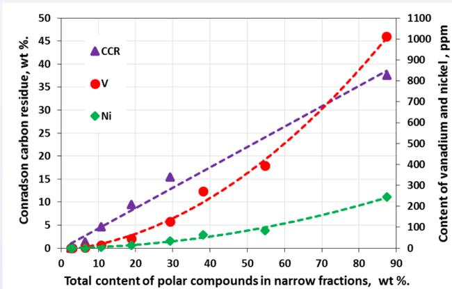
Figure 5. Content of CCR and metals versus total content of polar compounds in SFEF narrow fractions
