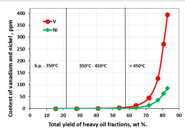
Figure 6. Vanadium and nickel concentrations of SFEF narrow fractions of heavy oil
