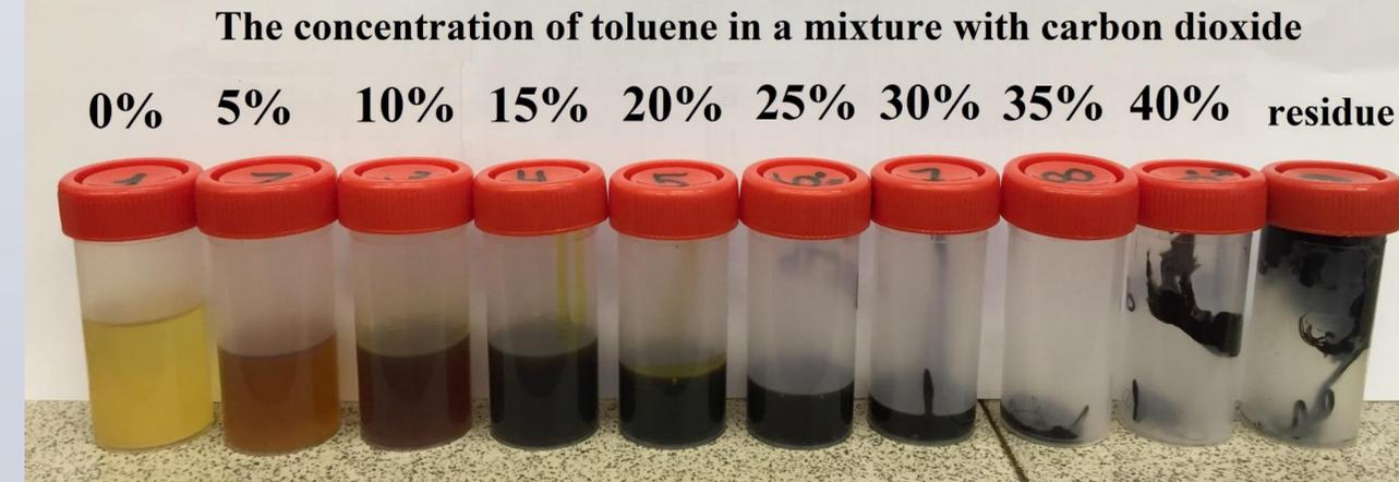
Figure 2. Narrow fractions of heavy oil obtained by SFEF using a mixture of carbon dioxide-toluene as a solvent
