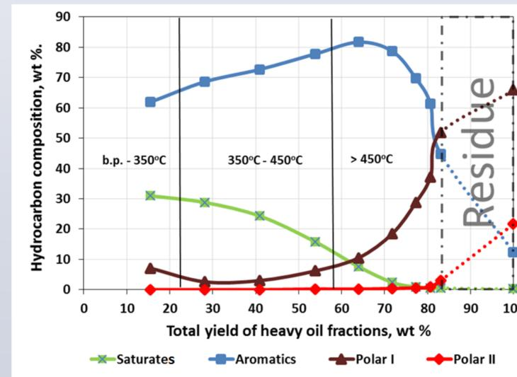
Figure 4. Saturates, aromatics, polar I and polar II percentages of SFEF narrow fractions of heavy oil
