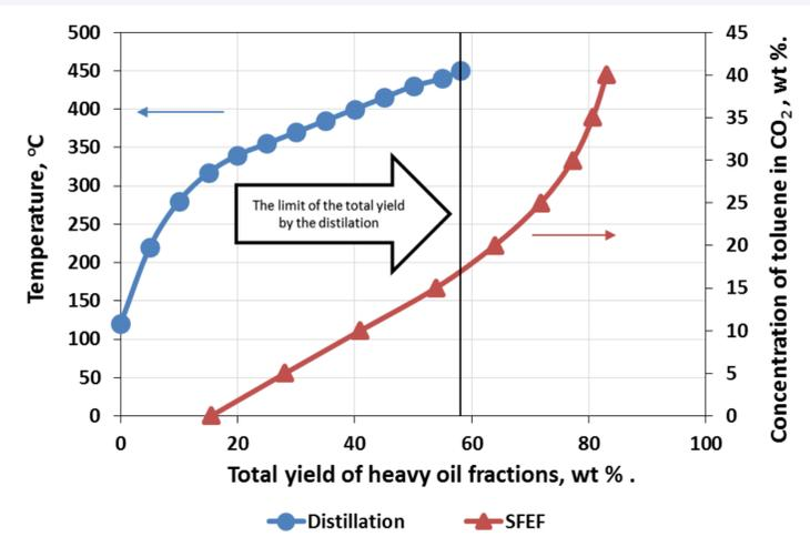
Figure 3. Comparison of the depth of the separation of heavy oil into fractions by the distillation method and SFEF
