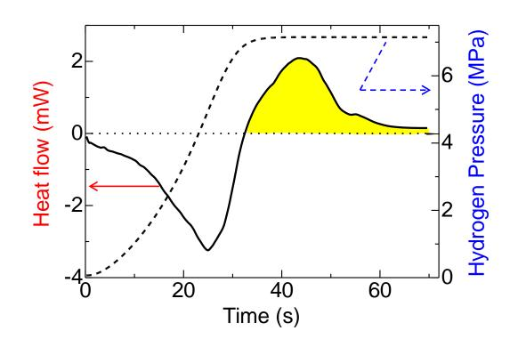
As hydrogen pressure was increased, an exothermic peak was observed; this trend is characteristic of hydrogen adsorption.
