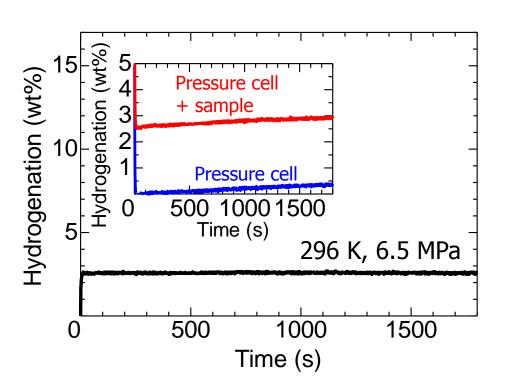
2.6 wt% hydrogen is **rapidly** adsorbed in the single-crystal material at room temperature.
