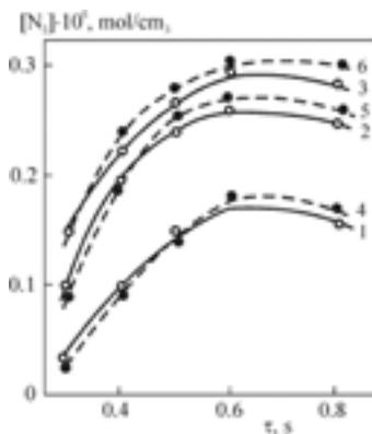
Figure 1: Kinetics of nitrogen fixation with hydrogen peroxide: molar ratio N<sub>2</sub>:30% H<sub>2</sub>O<sub>2</sub> = 1:1.6; 1 – 3 – T = 773, 823 and 873 K, respectively; 4 – 6 – theoretical curves at these temperatures
