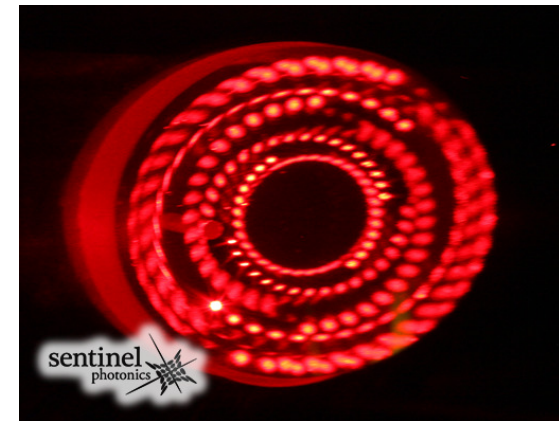
MPC dimensions: 17 x 6.5 x 5.5 (cm) Distance between the MPC mirrors: 12.5 cm
