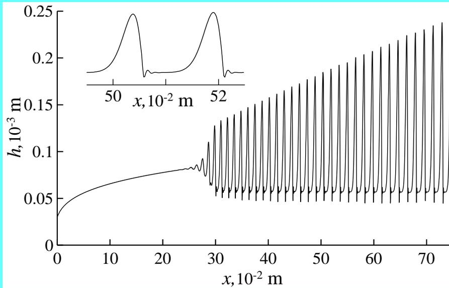
**Waves with a frequency **18 Hz**. Wave structure is shown in detail in the left upper part.**
