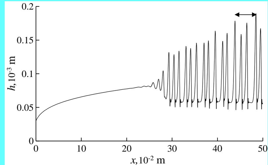
**Waves with a frequency of **6 Hz**. Double-arrow section corresponds to «wave length».**
