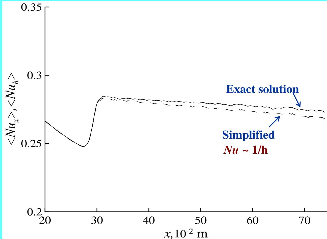
Dependence of time-averaged **Nusselt** number on **coordinate** at  $f = 18 \text{ Hz}$ ; solid line is **exact solution**; dashed line corresponds to calculation by **simplified formula**:
