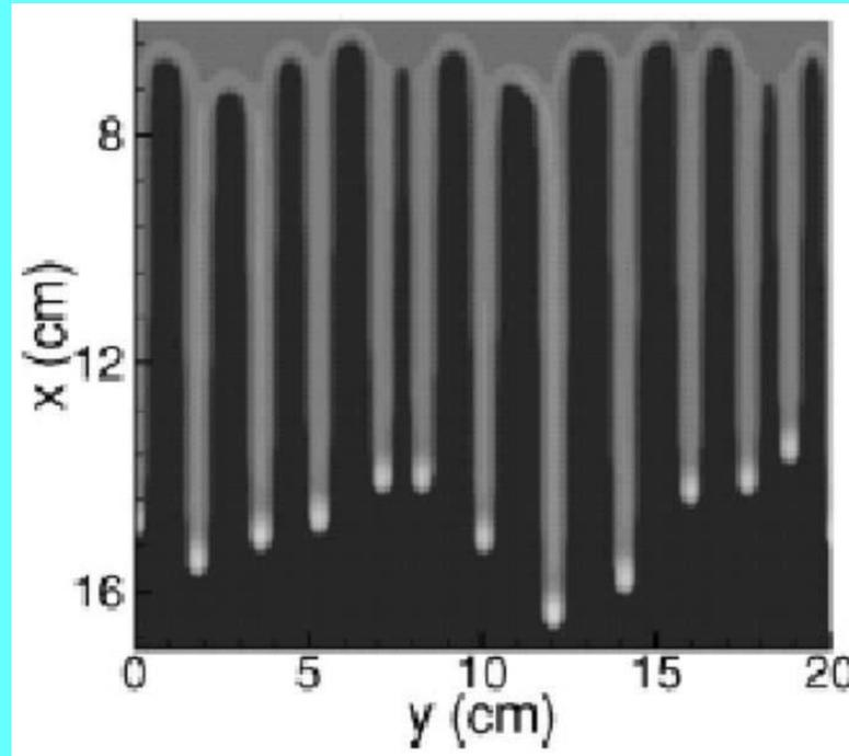
**Viscous film flow of water-glycerol solution (Johnson et al. 1999)**
