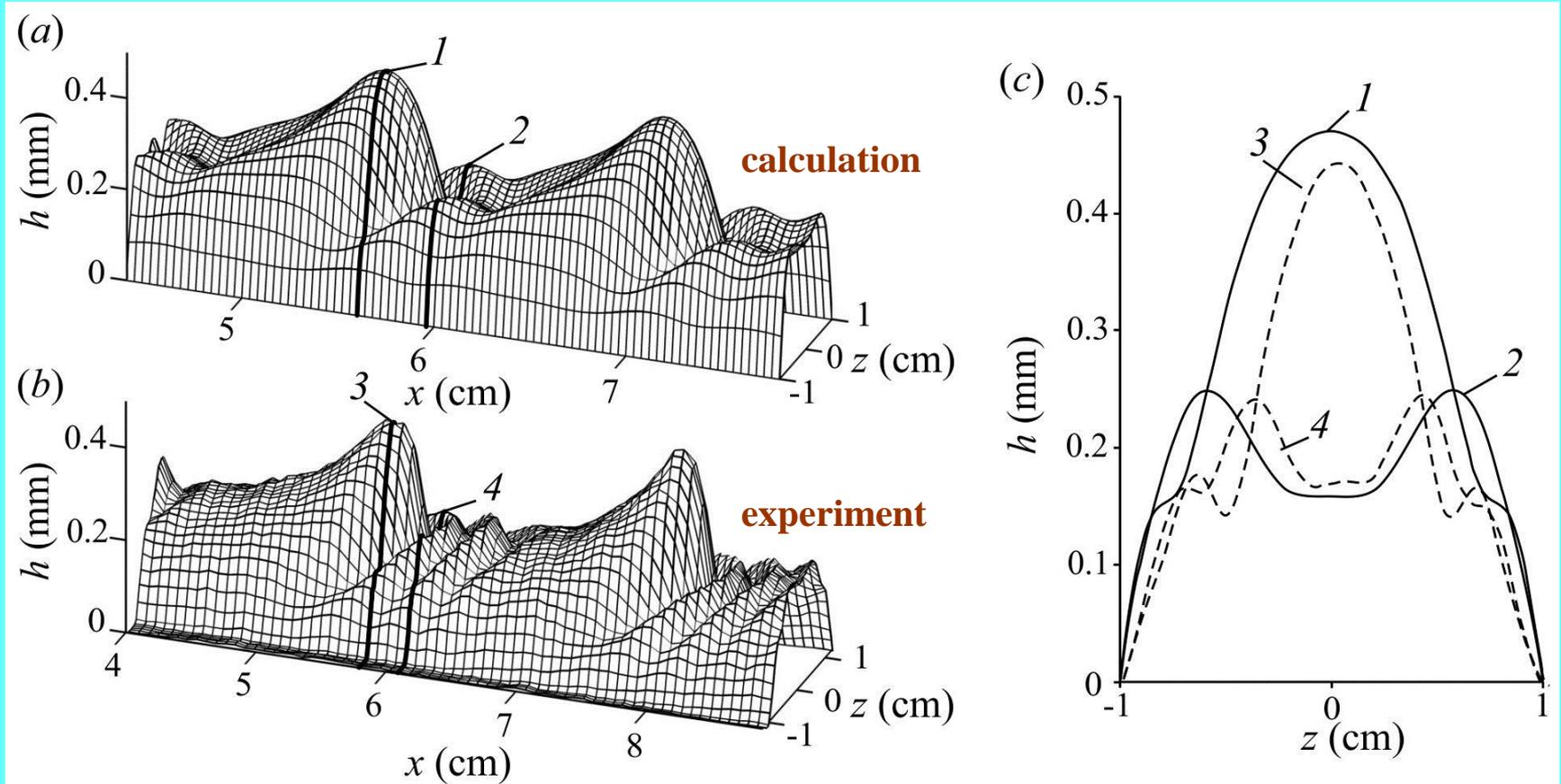
Shape of developed wave in **WGS** rivulet compared to the experimental data (Alekseenko *et al.* 2010) at  $Re_m = 36$ ,  $f = 23$  Hz.
