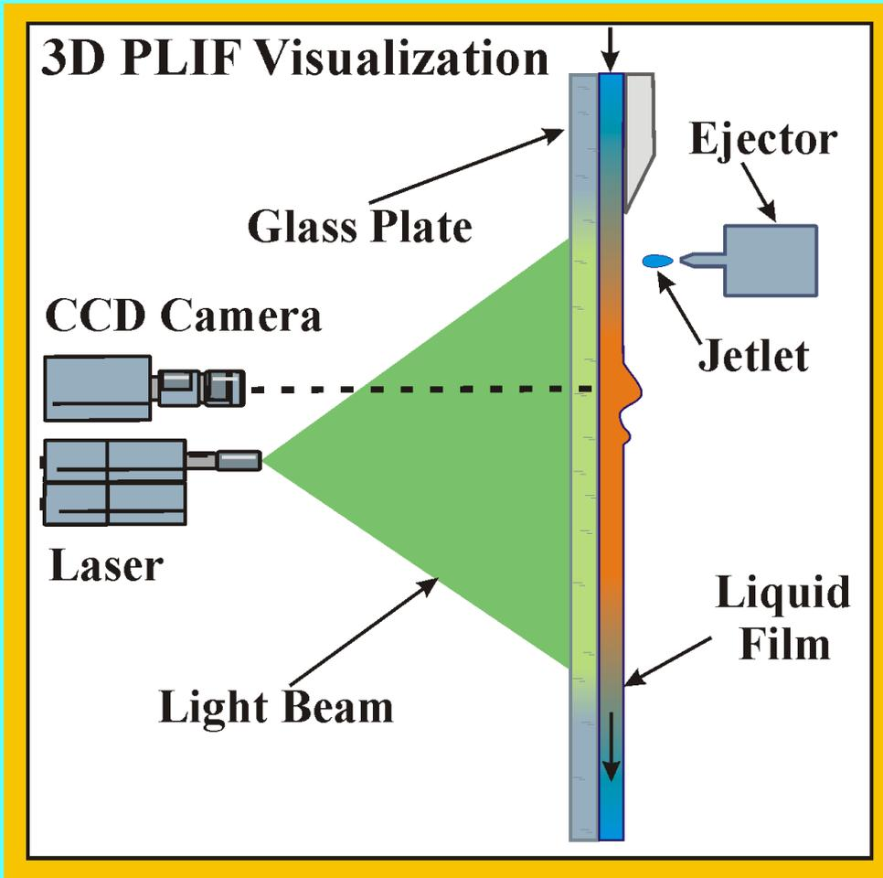
Measurement of 3-D distribution of liquid film thickness with **Planar Laser Induced Fluorescence** method (PLIF):
