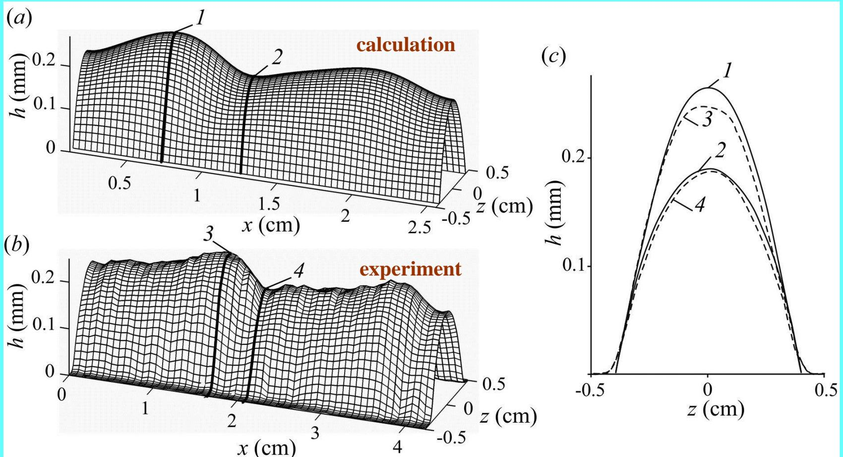
Shape of developed wave in **WGS** rivulet compared to the experimental data (Alekseenko *et al.* 2010) at  $Re_m = 10$ ,  $f = 15$  Hz.
