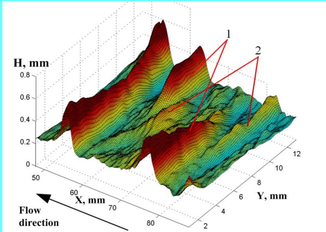
Appearance of **edges of primary waves** means that **not all the primary waves form full rings** around the circumference of the pipe.
