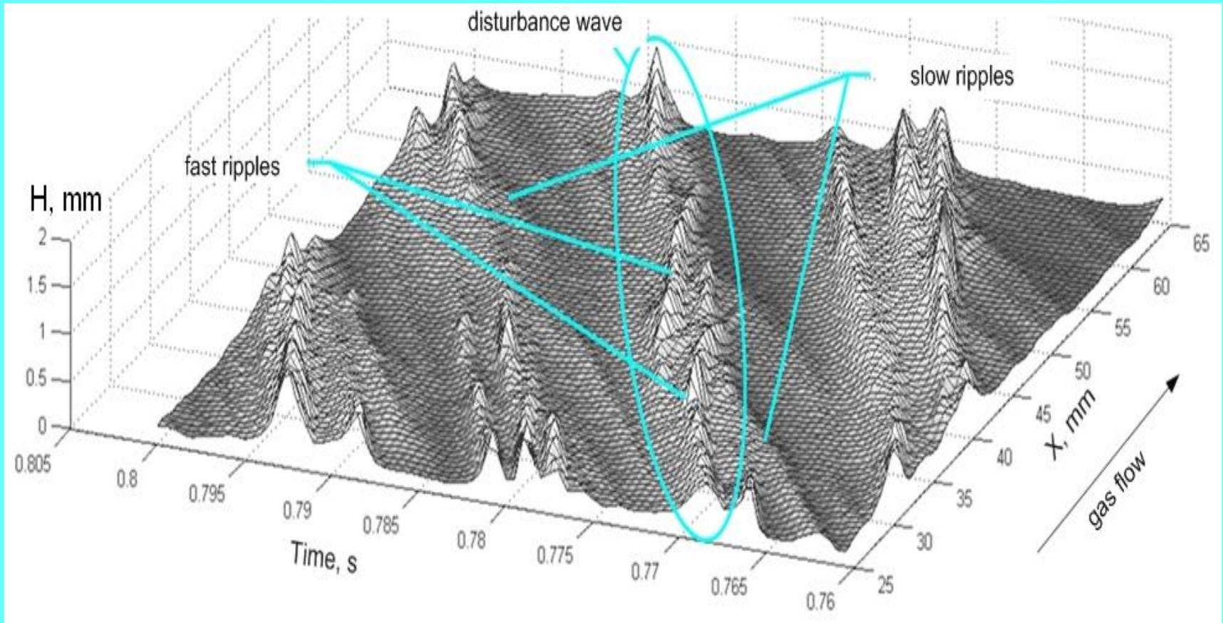
**Fast ripples on the disturbance wave and slow ripples on the residual layer.  $Re_L = 350$ ,  $V_g = 27$  m/s.**
