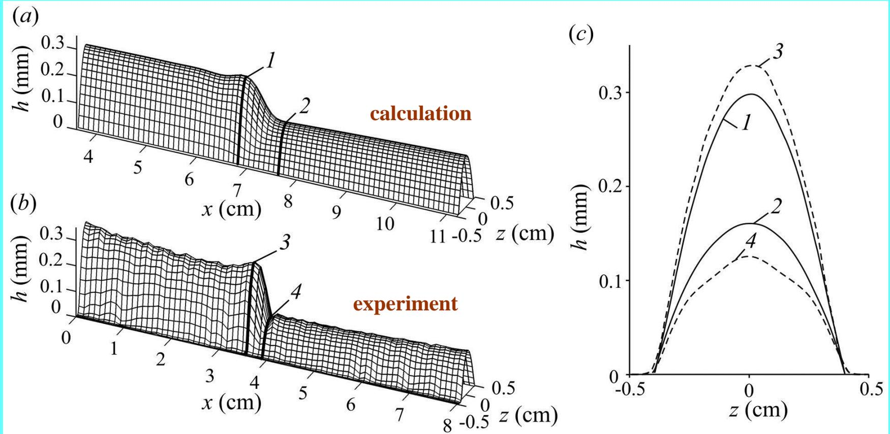
Shape of low-frequency wave in **WGS** rivulet compared to the experimental data (Alekseenko *et al.* 2010) at  $Re_m = 10$ ,  $f = 1$  Hz.
