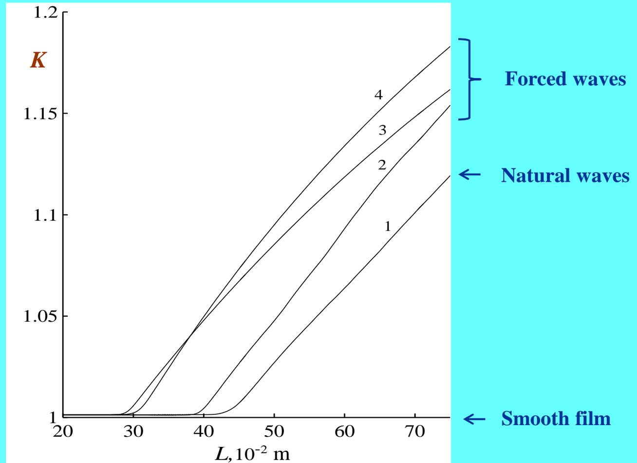
Dependence of the dimensionless integral **coefficient** of heat transfer enhancement  $K$  on the plate length  $L$ ; 1 – **natural waves**.
