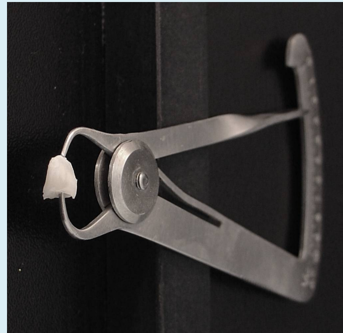
Dental metal thickness compass, ( Fara Dental, Germany ), used for (CrT) dimensions.
