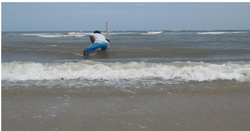
Plate 3.Wave breaker Height -Updrift
