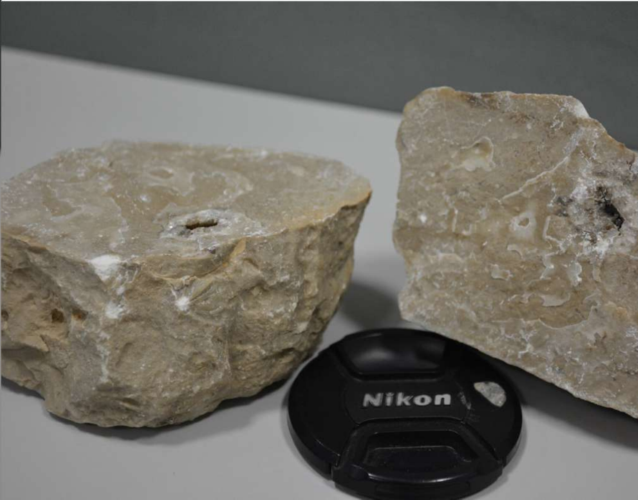
grey dolomitic limestone with cavity
