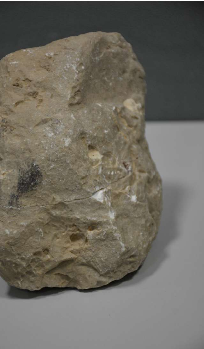
grey dolomitic limestone with cavity
