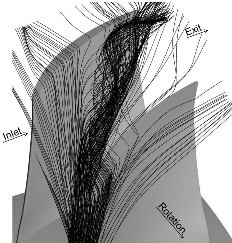
Rotor tip leakage flow
