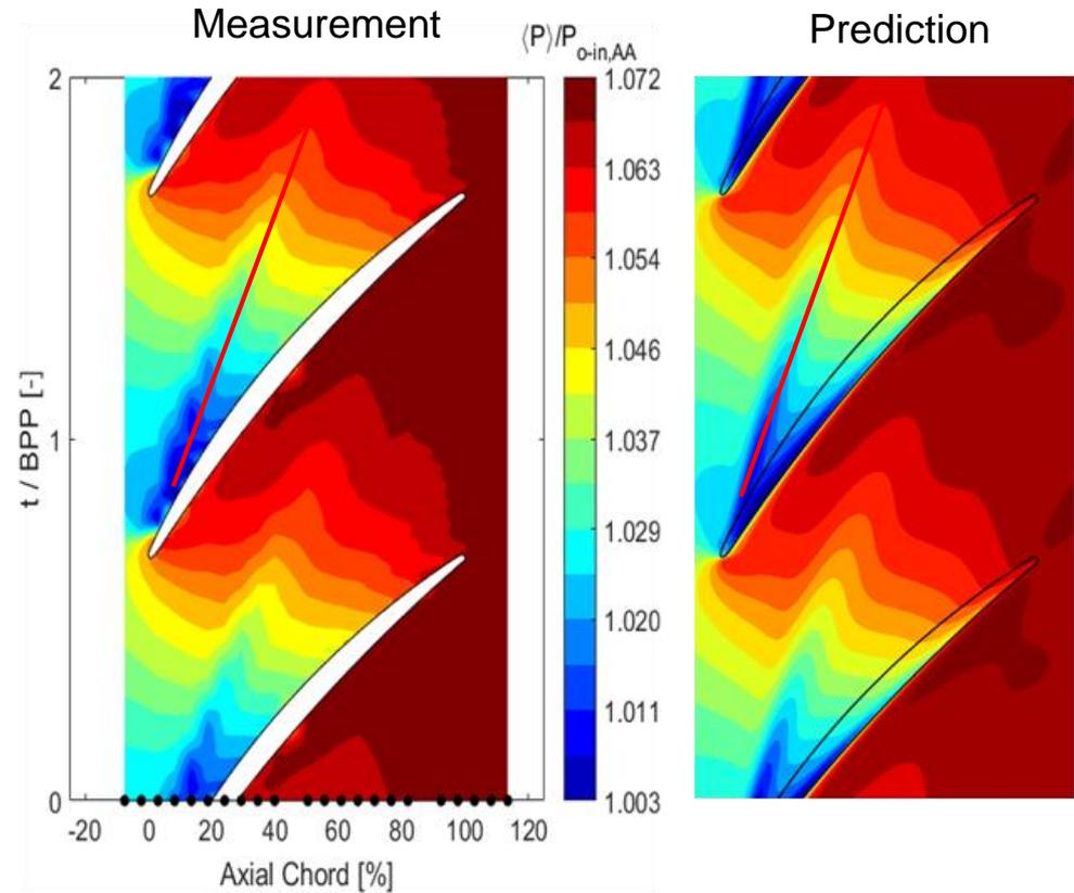
R2 casing time-averaged static pressure field (HL). Black dots show the positions of functional Kulites.
