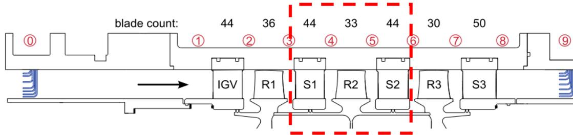
A thin slice at the mid span is used and three rows are included
