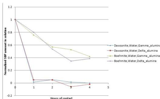
Figure1: UV-Vis results showing adsorption of soybean peroxidase in water by different phases of alumina from dawsonite and boehmite.
