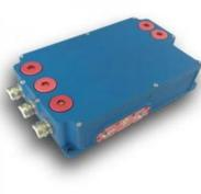
Generator Control Unit: Rhinehart Motion Systems RMS-PM150DZ Peak Power: 100 kW Continuous Power: 70 kW Continuous Output Current: 300 A Peak Output Current: 500 A
