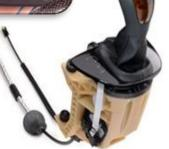
Shift Lever Operating DC Voltage: 12 V Communication: CAN
