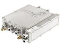
Motor Controller: TM4 MΦTIVE: Series C060 Operating DC Voltage: 220-400 V Minimum Operating DC Voltage: 180 V Accelerator Pedal Operating DC Voltage: 12 V Sensor: Programmable Hall Effect SensorType: Dual Potentiometer
