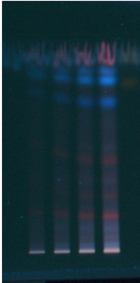
HPTLC Video image of E. canadensis at 366 nm in chloroform: methanol(9:1 v/v )
