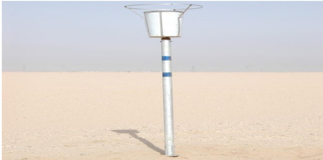
Dust collector (source: Reheis, 1 995 with some modifications).
