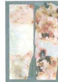
Figure 4.4: Degraded rubber pieces after burial in sewage sludge
