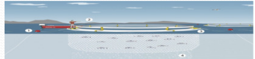
1. The cage is moored to the ocean floor 2. Fishmeal based feeds are added to the cages 3. Buoyant tubes keep the cages afloat 4. Fish faeces and waste fall through the cages
