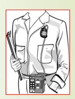
Major components of fine particulate matter sampler with a flow rate of 4 Lpm, with impactor developed by the School of Public Health at Harvard, adapted for individual use at LPAE.
