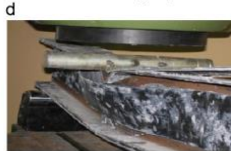
d mixed mode failure (with debonding at compression and tension flange and on web)
