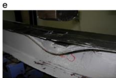
e compression flange debonding
