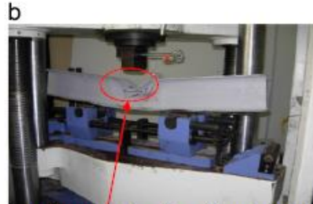
b ductile symmetric collapse (forming deep kink and web crippling)
