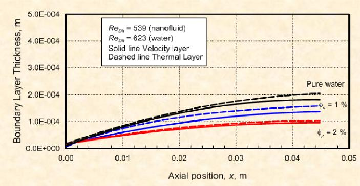
Thermal and Velocity boundary layer thichness along the micro-channel flow direction for different Al<sub>2</sub>O<sub>3</sub> concentrations (m = 5.49 g/s, Q=300 W).
