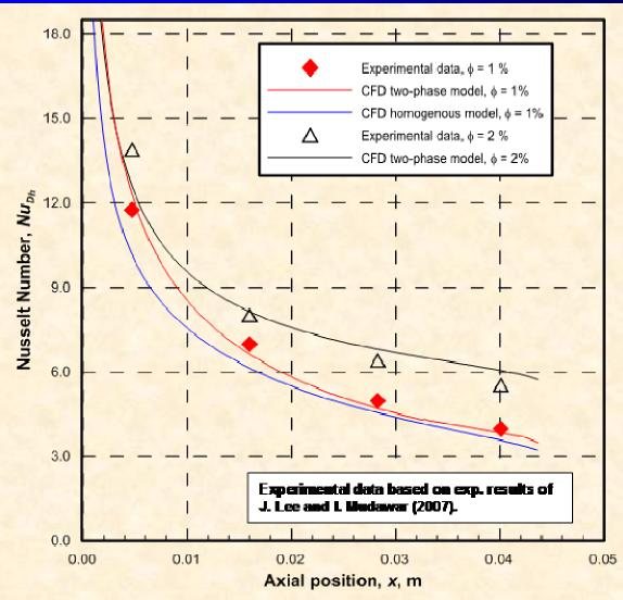
Variation of local Nusselt Number along the micro-channel flow axial direction for different  $Al_2O_3$  concentrations. (m = 5.49 g/s, Q=300 W)
