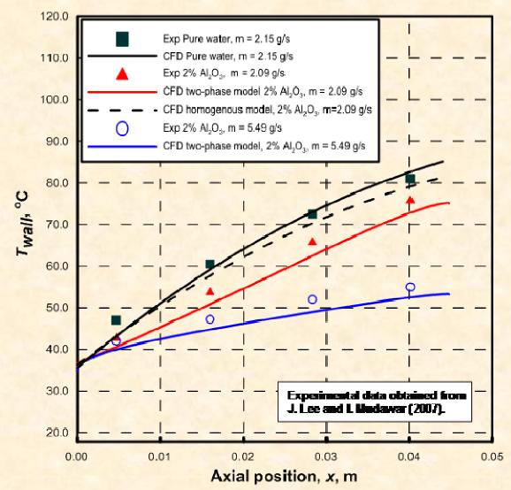
Variation of wall temperature along micro-channel axial flow direction at symmetry plane for different flow rates. (Q=300W)
