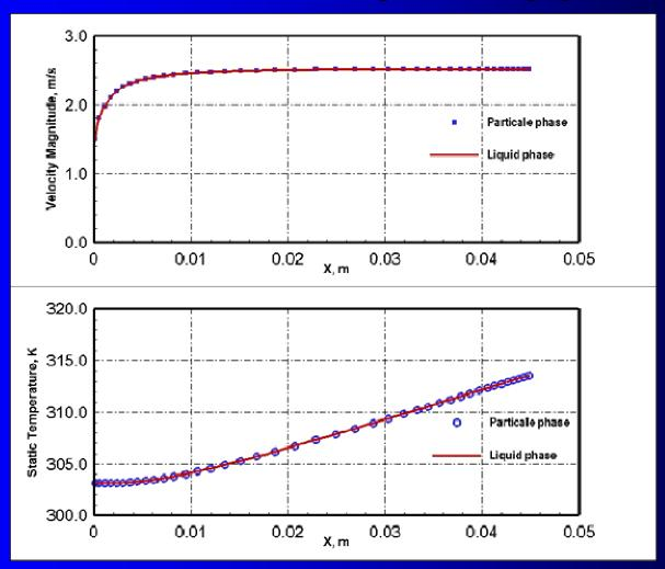
Velocity and temperature profiles for the phases of 2% Al<sub>2</sub>O<sub>3</sub>/water nanofluid using the Eulerian-Eulerian two-phase flow model for Re=530, m=5.49 g/s, and heat input (Q) = 300W.
