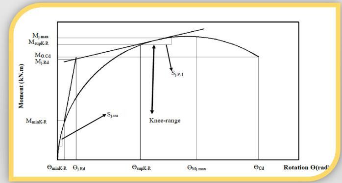
• The rotation and the bending moment (M) are predicted by using displacements of the beam as well as multiplication of the distance between the load application point and beam end bolted to the column ( $L_{load}$ ), respectively:
