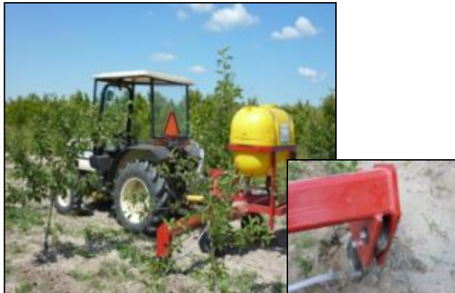
Injecting a preparation below soil surface near plant roots
