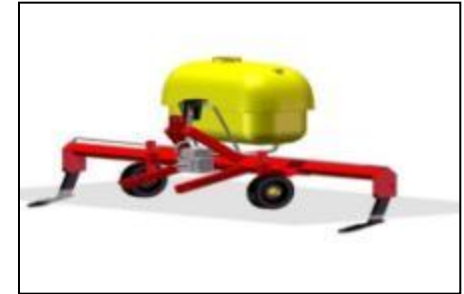
Feeder for applying mycorrhizal preparations under soil surface close to the root system
