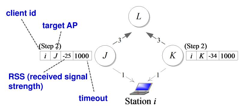
(a) Both APs J and K send the station *i* a Probe Response (step 1), record the information in their respective association tables (step 2) and broadcast the recorded information to the LAN (step 3.) This enables association tables at different sites to accumulate same entries.
