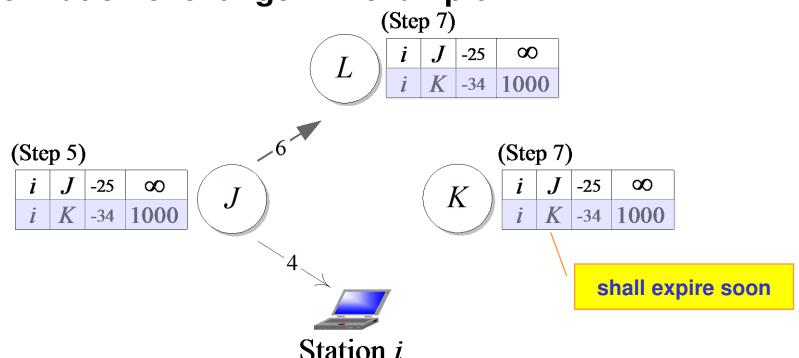
(b) AP J accepts and sends the station i an Association Response (step 4), resets the entry with index (i,J) to have infinite Expiration Time (step 5), and broadcasts the event of association to the LAN. Upon receipt, APs update the corresponding entry accordingly in their maintained tables (step 7.)
