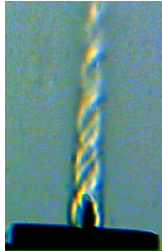
Fig. 4. Structure of supersonic jet when b=3 mm, annular nozzle diameter is 3 mm, slit a is 1 mm, pressure in pre-chamber is 0.6 MPa. Here Toepler method is used (provided in MSU SRI of Mechanics)
