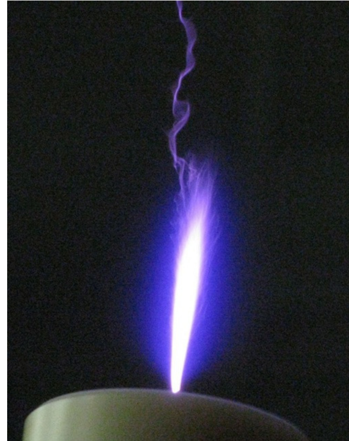
Fig. 9. 1.4÷1.6 MHz HF field is applied at the cone . All other details of the dynamic emitter are dielectric. The pressure is as for Fig. 12.
