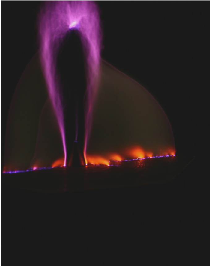
Fig. 8. Antenna disposed on 10 cm over top of the flow of grounded nozzle. 1.4÷1.6 MHz was supplied on antenna. Pressure in pre-chamber is 0.6 MPa. Without gas flow – dark frame
