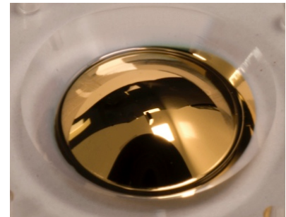
200nm gold coating (Chemical Vapor Deposition)
