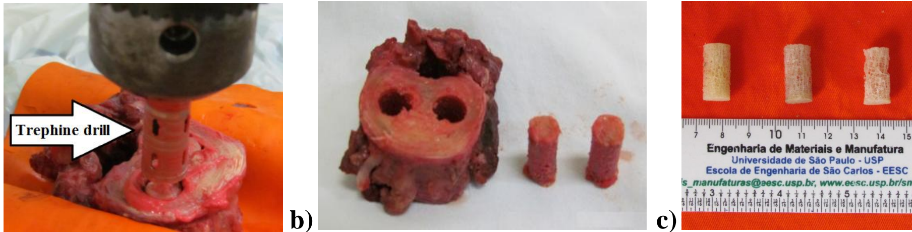
FIG. 04 – a) Vertebral body penetration through the trephine drill; b) Cylindrical specimens of trabecular bone; c) Proof bodies (20 by 10) mm without bone marrow of L 1 region, classified as normal, osteopenic and osteoporotic
