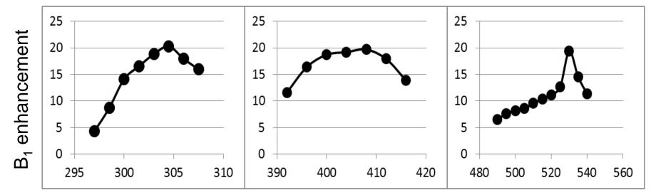
The tuning frequency of the inner micro-LC circuit (MHz)
