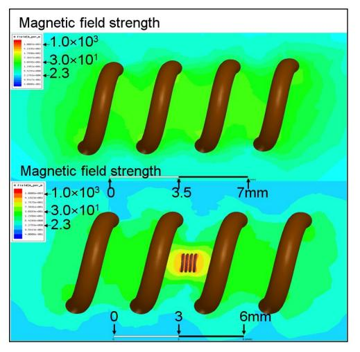
The magnetic field with the inner micro-RF coil resonator is 20 times that without the inner micro-RF coil resonator.
