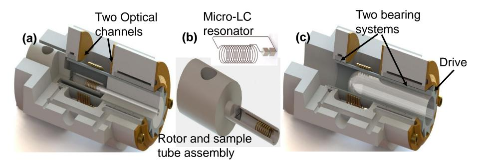
(a) Small samples of variable sizes; (b) Switchable plastic plug with a micro-LC resonator for enhanced sensitivity; (c) Large biological objects.
