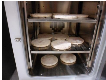
Placing Materials inside a Circulating oven at 90\pm 2^{\circ}\text{C} for 1 hour
