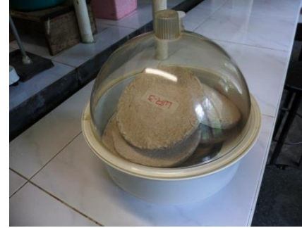
Cooling down of Material samples inside a Desiccator at Room Temperature for 30 minutes
