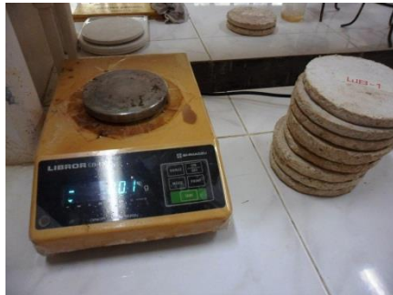
Weighing of Materials
