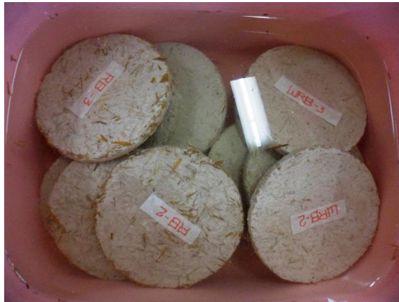
Soaking of Material Samples in Water for 24 hours
