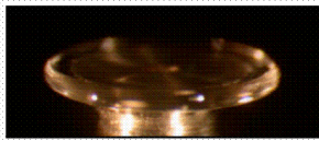
Calcium fluoride resonators that have Q=2 \times 10^{10} .
