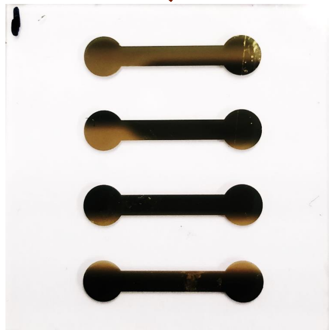
Plasma corona treatment of PDMS surface and 4 channel SPR sensor
