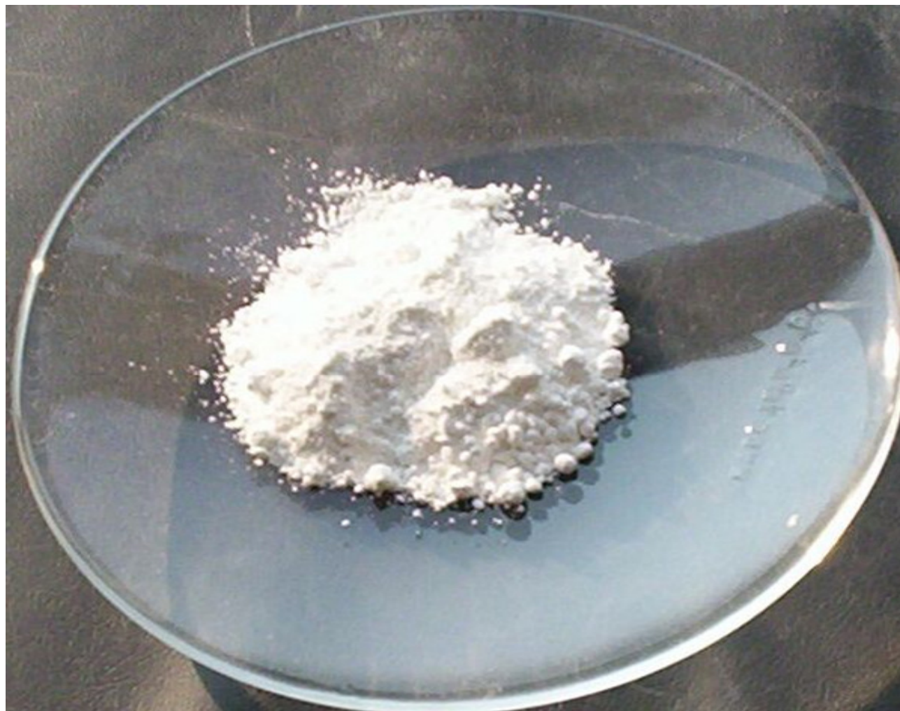
Fig 3. Zinc oxide nanoparticles powder (provided from nanomaterial Co. Huston, TX, USA. Purity > 99.99%,
