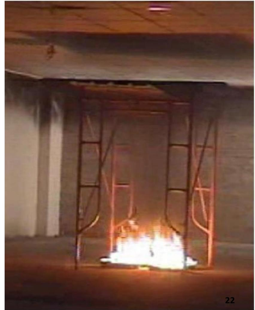
Diesel pool fires were set up at floor level at about 9m away from the north end and in the middle of the two sidewalls
