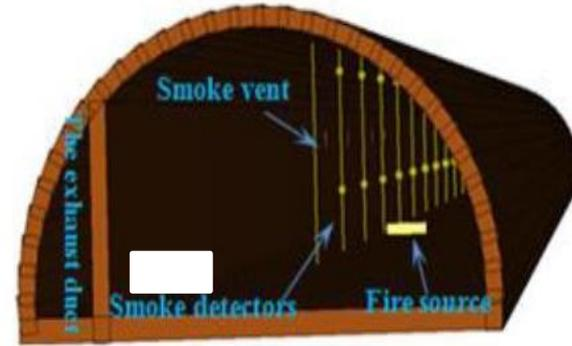
Fig. 1. Model configuration of the tunnel.
