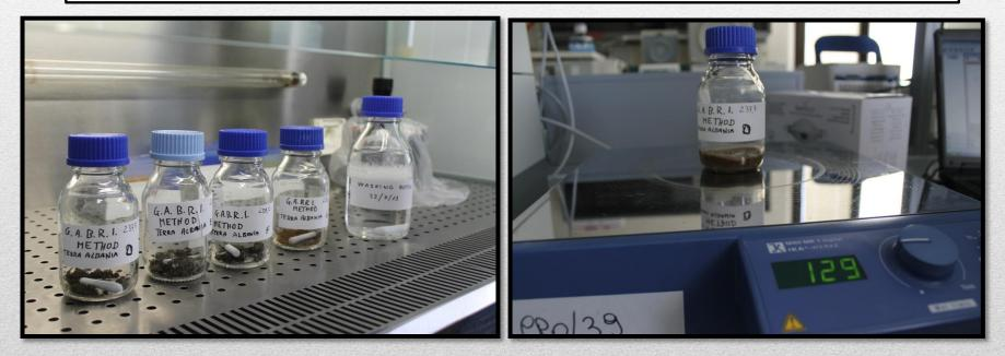
After washing in magnetic stirrer for 30 minutes, the suspension was centrifuged for 5 minutes at 2000 rpm and the supernatant incubated for 20 minutes at 64°C.
