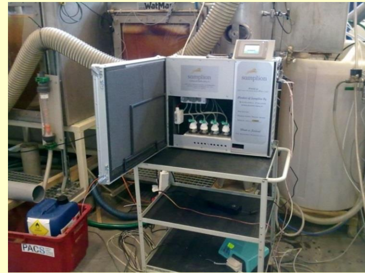
PMEU with Automated Sample Collection System
