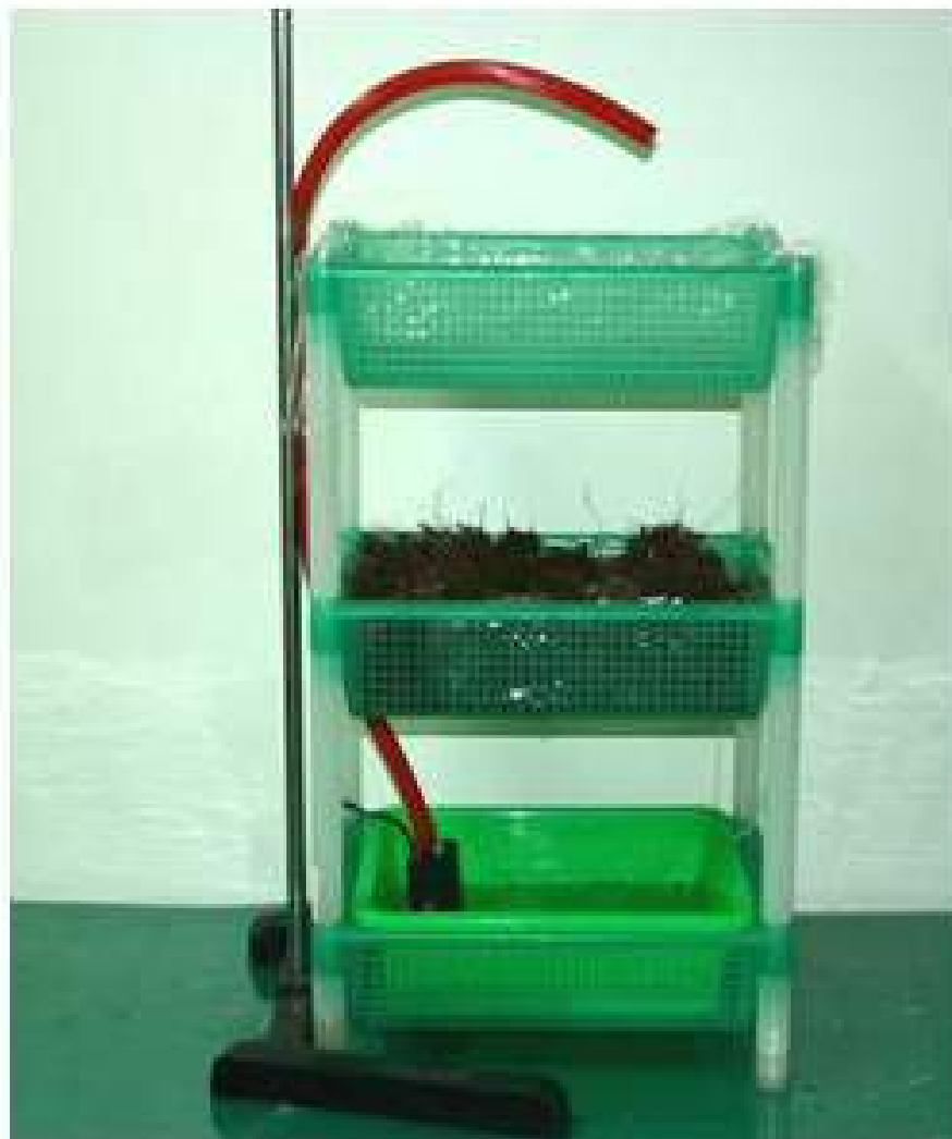
Figure 2. The leaching apparatus system: Upper part is a plastic tray, 55×40×15 cm with numerous needle-sized holes (2 cm between holes) was filled with tap water, which dripped through the holes to make an artificial raindrop, middle part is the same as upper tray, was filled with chopped plant material/organic matter to receive the artificial raindrop from upper tray, lower part is a plastic tray, like that of upper and middle tray, without holes to receive plant leachate from middle tray. The pump re-circulated the water from lower tray to upper tray
