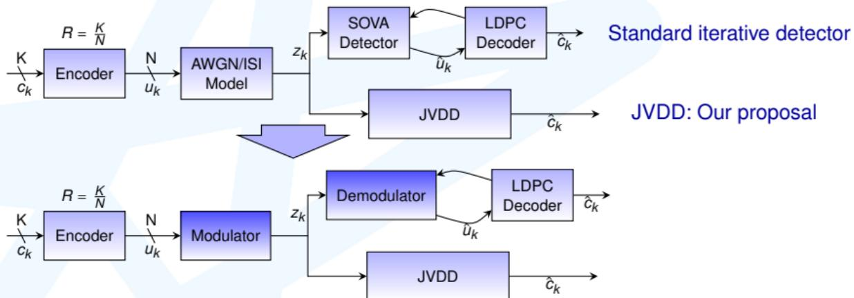
Joint Viterbi Detector/Decoder (JVDD) is a higher performing alternative scheme to existing iterative detection schemes
