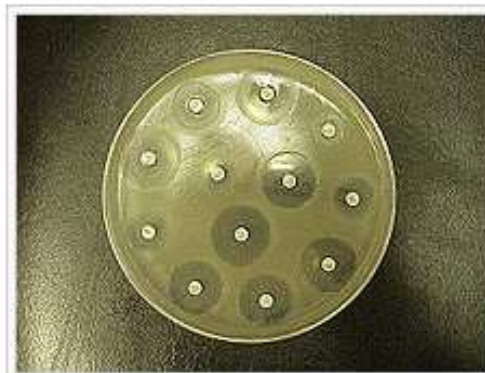
In Kirby-Bauer testing, white wafers containing antibiotics are placed on a plate of bacteria . Circles of poor bacterial growth surround some wafers indicating susceptibility to the antibiotic.
