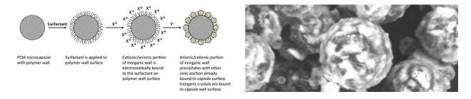
To demonstrate the silver coating is in fact, coating the PCM capsules, SEM images are provided above in **Figure 1**. In the SEM images, silver appears brighter and white, as the electron density of silver is much higher than that of the organic microcapsule wall. From this, the silver coating is very well attached to the PCM microcapsules.
