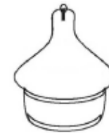
T 5 Spherical trap with bottom hole and rubber septum
