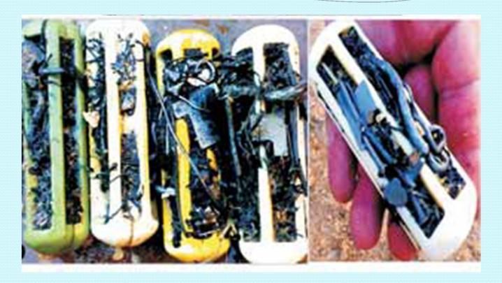
Complete filling of cage magnets with foreign bodies. The magnetic power of the retrieved reticular magnets was similar to the new one
