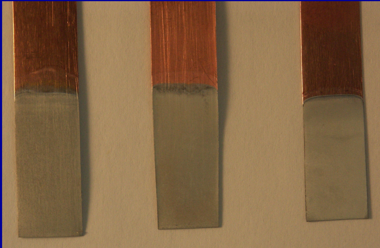
Fig.: Electrowon Zn-Pb on copper substrate from the electrolyte produced by dissolving the EAF dust in 1 ChCl:2 urea ionic liquid at 60°C
