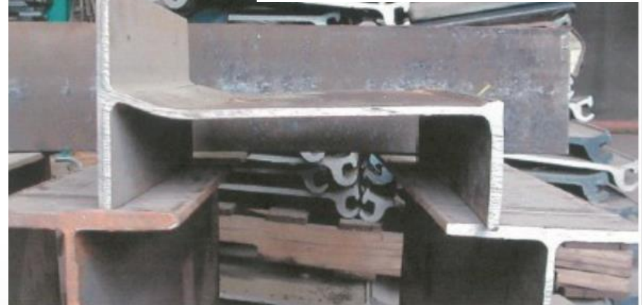
Wide-flange shape with buckled web and one-half of flange broken off (photo courtesy of Nucor-Yamato Steel Company).
