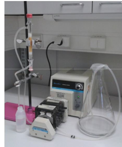
Fig. 7. Column apparatus for tests on mining wastewater.
