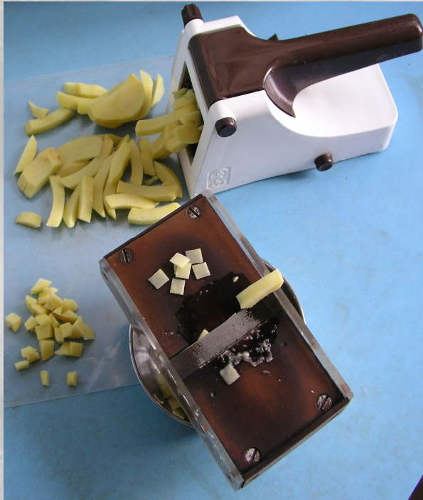
Potato sample cut from inner parenchyma 100 g, 10x10x1.5 mm
