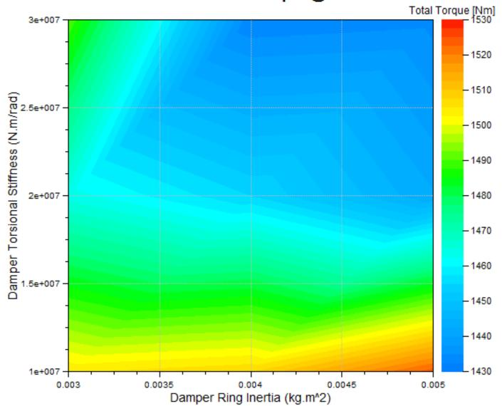
The highest magnitude of torsional torque occurs at fillet of web8 . it can reach more than 1500 N.m
