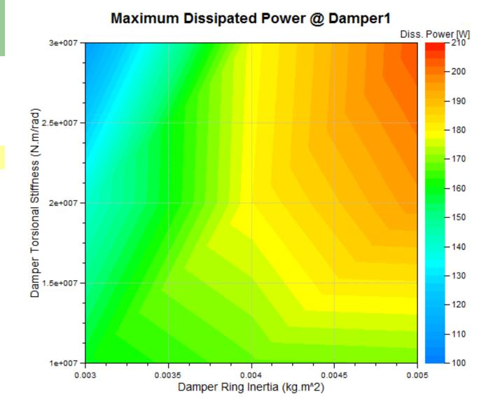
The biggest power dissipation (210 W) occur at right and upper side. Too much dissipated power can wear elastomer material of TV damper.
