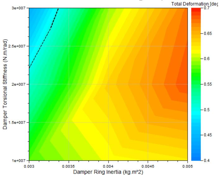
The most deformation on TV damper occurs at 2\*107 stifness and 0.005 inertia value as smilar with dissipated power graph
