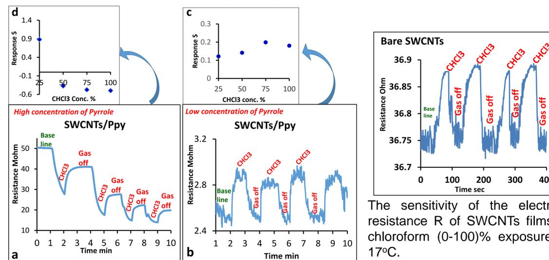
(a&b) The sensitivity of the electrical resistance  $R$  of SWCNTs/Ppy films to chloroform (0-100) % exposure at 17°C; (c&d) The device sensitivity  $S = (R - R_0) / R_0$  as a function of chloroform. Fig (a) shows the swelling effect of pyrrole on the gas response.
