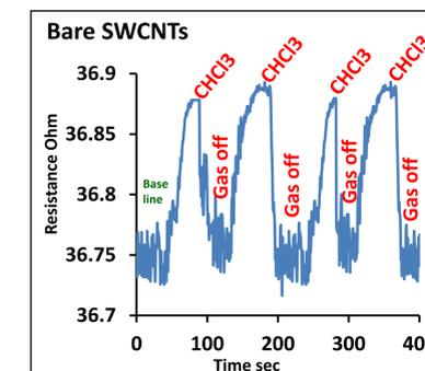
The sensitivity of the electrical resistance  $R$  of SWCNTs films to chloroform (0-100)% exposure at 17°C.
