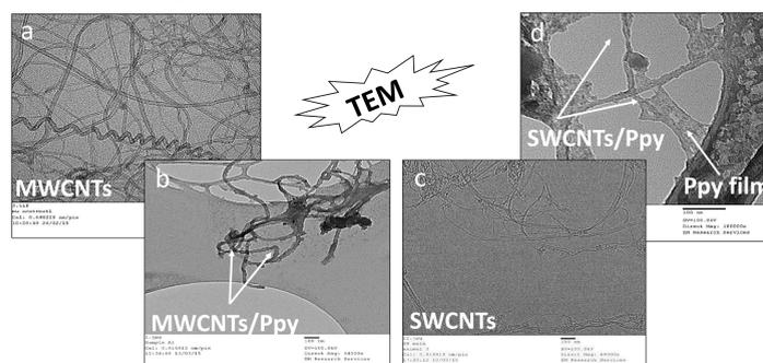
TEM images of (a) multiwall carbon nanotubes before coated by Ppy (Mag 130000x), (b) hybrid MWCNTs (Mag 64000x), (c) bare SWCNTs (Mag 64000x), (d) SWCNTs after templated by Ppy (Mag 1800000x).
