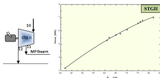
For the back pressure steam turbine STGII, The generated power increases linearly to achieve about 7 MW for a HP steam mass flow rate of about 82 t/h.
