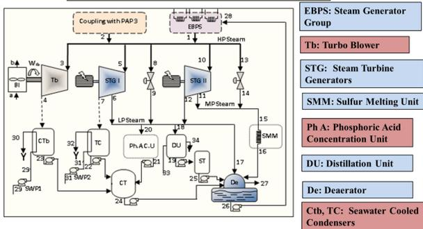
The STGI is with extraction and condensation, while the STGII is with extraction and back pressure turbine
