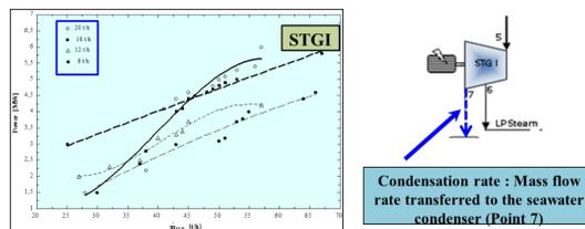
The generated power increases gradually with HP steam mass flow rate. For HP steam flow rate less than 35 t/h the generated power is not significantly affected by the condensation rate.
