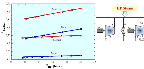
The energy and exergy efficiencies increase linearly with the pressure of steam. For the explored ranges of pressure, the energy efficiencies increase of about 1.37 % and 8.8 % for STGI and STGII respectively.
