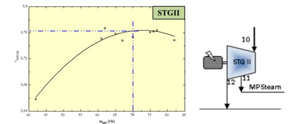
The exergetic efficiency increases sensibly with HP steam mass flow rate to reach a maximum value of about 75.5 % for a mass flow rate of about 73 t/h. That can be considered as an optimum value for the STGII supply.
