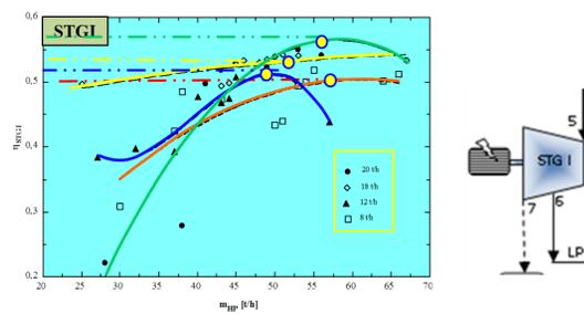
The exergy efficiency increases with HP mass flow rate to reach maximum values as follows:
