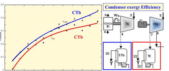
Increasing the seawater temperature from 12 to 24 °C leads to an increase of the exergy efficiency of about 6 times for the turbo blower condenser CTb and 14 times for the turbine condenser TC.
