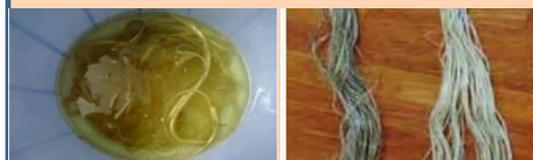
Fig.3 Treatment of Fiber in 2% NaOH solution
