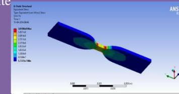
Fig.12 Equivalent stress of the composite specimen
