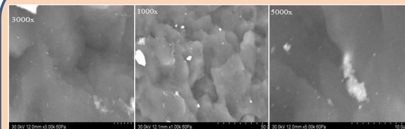
Fig.13 SEM analysis on the surfaces of the polypropylene resin with Kenaaf fiber shows the fine distribution of fiber in resin in matrix with the required resolutions .
