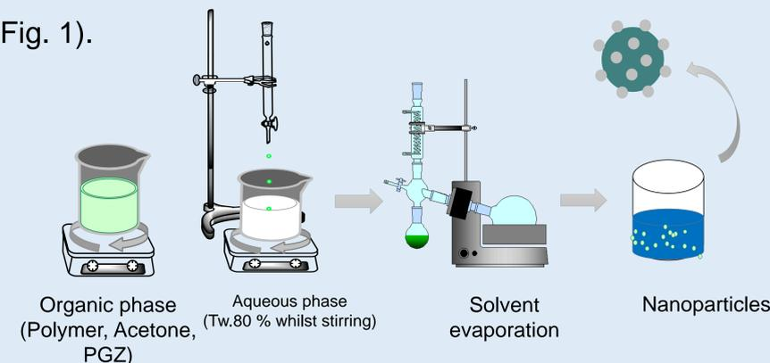
Fig. 1 : Elaboration method of PGZ-NPs
